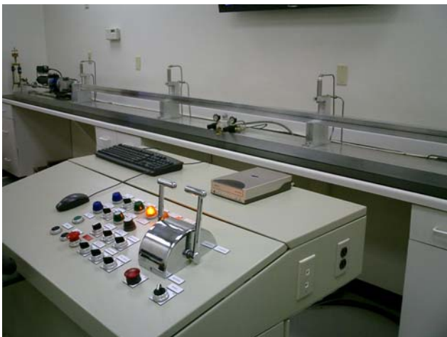
Figure 9: Physical Simulator of the Directional Drilling Process Used for Training.
