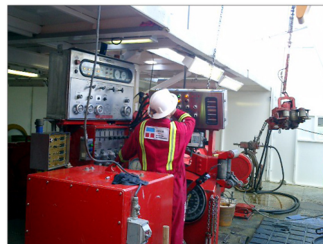
A top-drive technician tests the Slider equipment soon after installation on a land rig working for Anadarko in Canada.
